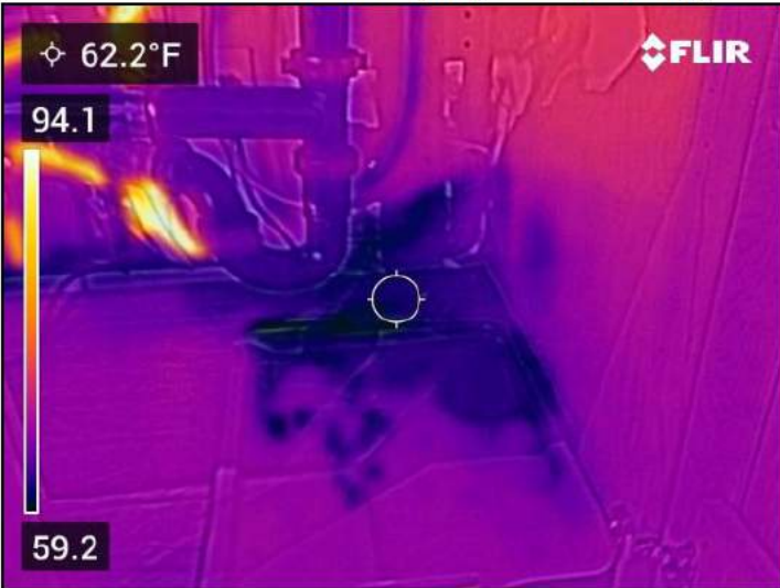
Leak from the sprayer
